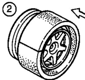
Mount the foam filler over the wheel and adjust.
