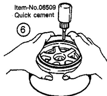
Lift the tyres, which sit close at the wheel on this place where you have to glue, so that the Super Glue flows between tyre and wheel. Tyres which don't sit close at the wheel on this place where you have to glue, we recommend to glue the tyre point by point with the wheel. Press tyre and wheel together at the place you have glued them.
