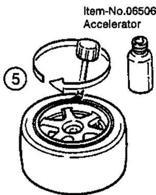
Adjust the tyres and make sure that the edge is exactly in the groove. Spread the Activator Fluid 06506 in the gap between wheel and tyre.
