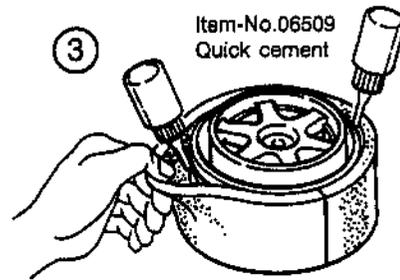
Glue the foam filler with the Super Glue extensive to the wheel. It is important that you glue the edges properly, otherwise it's possible that they loosen when you mount the tyres.
