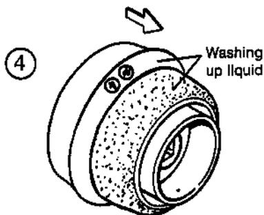
Apply washing up liquid on the marked side of the tyre and mount the foam filler which is glued tight to the wheel. Wipe the rests of the liquid away.
