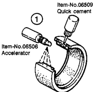
Before you glue the foam filler together, put it over the wheel and check its length, if necessary shorten it. Glue the foam filler wide/narrow together. Spread the No.06506 Activator Fluid on the one side and the Super Glue on the other side. Instead of Super Glue you can also use contact adhesive. Then press both sides together.
