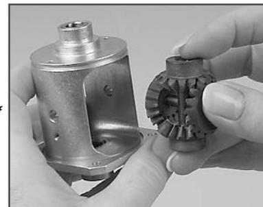
The FG Mounting tool 8505 guarantees an essential easier mounting of the diff. bevel gearwheels or rather of the complete package.
